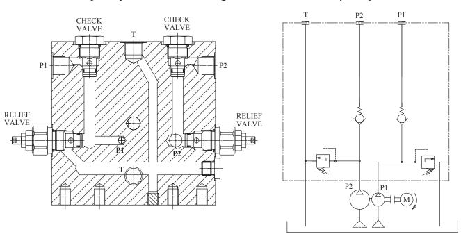
The W85A series power pack is designed for applications that need two independent hydraulic power supply,but only use a single A.C. motor.
